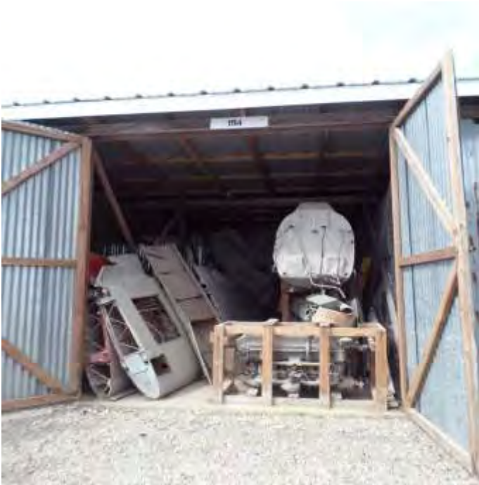
PT-19 parts including wings, center sections, Fuselages, tail feathers and a crated up engine
